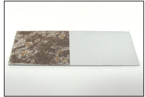
Salt fog test in action – showing the strong resistance of CORIUM 78 against corrosion and rust formation on the right
