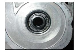
Chlorinated additives attack rubber and soon cause irreparable damage. Moisture such as condense, when combined with the chlorides, causes chemical reactions to take place, resulting in the formation of acid. The acid attacks the metal as well as the seals and this accounts for the leaks and corrosion found in transmissions.
