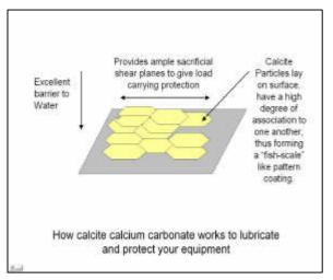
This technology has inherent advantages without the use of added performance additives. Omega 78 does not require the use of heavy metals, sulfur, chlorine compounds or other EP additives, to give the high EP/AW performance.
